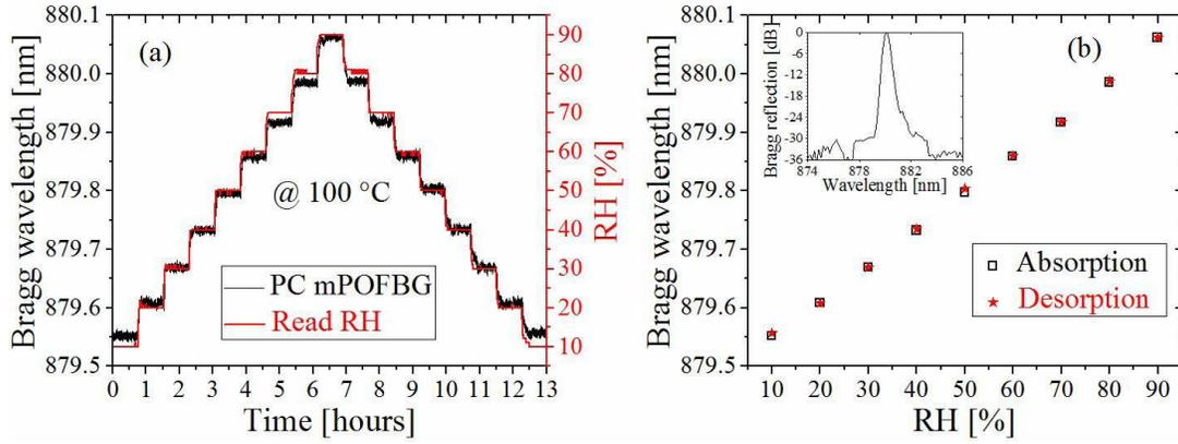
Fig. 3. (a) Measured humidity response at 100 °C of the PC mPOFBG. (b) Corresponding stabilized humidity response of the PC mPOFBGs at 100 °C. Inset: Normalized Bragg reflection spectrum of the PC mPOFBG.
